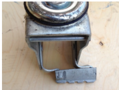
Foot pedal distortion as a result of a significant frontal impact; it is likely the top plate and bearing will be distorted as well.
