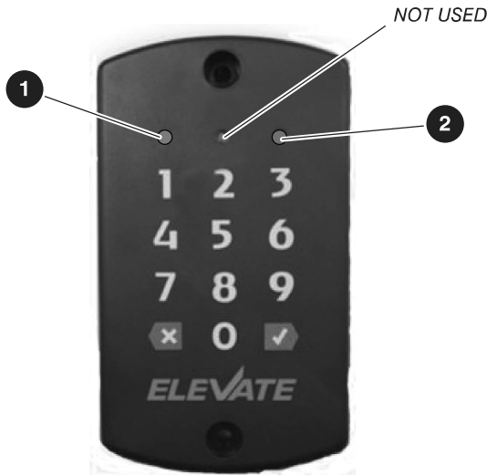
Figure 06 Keypad of the access control unit
