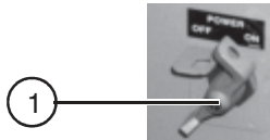
Figure 2-1. Main Power Disconnect Switch
